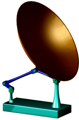
Figure 4: Radar antenna pitching mechanism.
